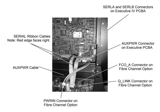
Figure 6-14 Detail of Connections (Executive IV PCBA Shown)
